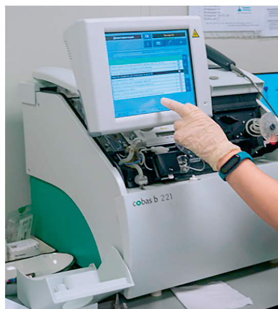
Fig. 6. Multiparameter analyzer of blood gases, electrolytes, oximetric parameters and metabolites Cobas b221 (Roche, Switzerland). (Photos from the official website of the I.I. Dzhanelidze Research Institute of Emergency Medicine)
